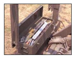
The steel toolbox upgrade kit replaces the plastic toolbox supplied as OEM equipment on US Army M1022-A1 Dolly Set Mobilizers. Field experience with the M1022-A1 system has resulted in reports of damage to the plastic toolbox during normal operations.
