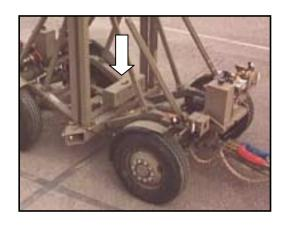
The dimensions of the new toolbox (32-in. long x 8.5-in. wide x 9.5-in. tall) present a lower profile than the plastic box while maintaining sufficient capacity for all M1022-A1 required items. The lower profile box does not interfere with any dolly set operation.
