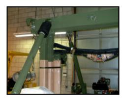
The Protective Bellows for the M1022-A1 Dolly Set Lift Cylinders (and CLT Dolly Sets) provides protection to cylinder rods from environmental conditions such as dirt, corrosive elements and blowing sand while dolly sets are in service or in storage.
