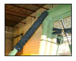
The Protective Bellows are custom designed for the M1022-A1 Dolly Set Mobilizer to provide maximum protection when the lift cylinders are fully retracted (unit on ground), halfway extended (normal ride height), or fully extended (high end-lift for aircraft loading).
