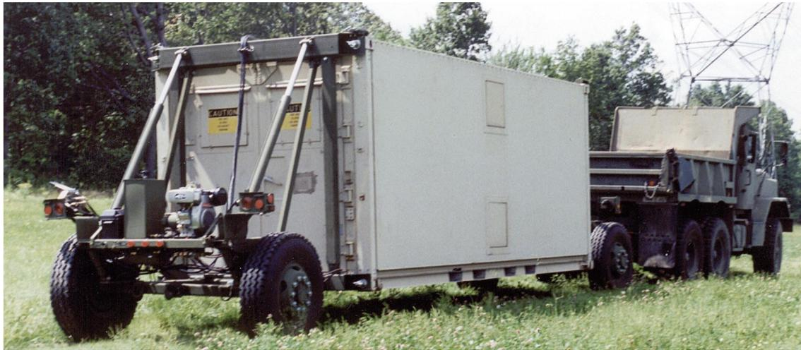
connected to a shelter, the dolly set can be coupled together as a 4-wheel trailer (in tandem if desired) for transport by road, rail, ship or air.
